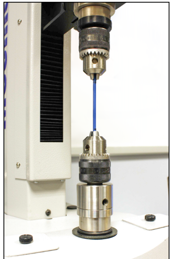
▲ Upper and lower 'key-operated' 3-jaw Chucks shown fitted to Helixa
