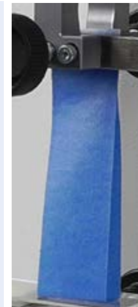
◀ Test Plate (PDV13016-A) shown with 25 mm strip being held in Upper Grip (Mec227-BG50)
