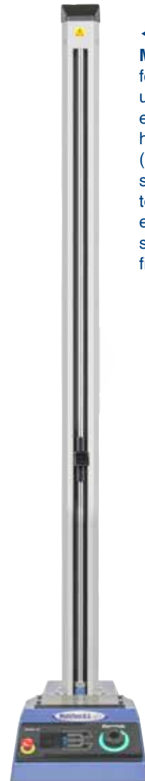
◀ MultiTest 1-dV for tension and compression applications up to 1 kN. The long column height of 1416 mm (56"), makes the MultiTest 1-dV a preferred choice for the elongation testing of moderately elastic materials and products
