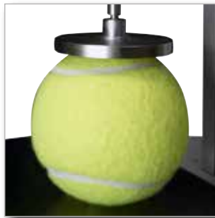
Tennis ball compression test
