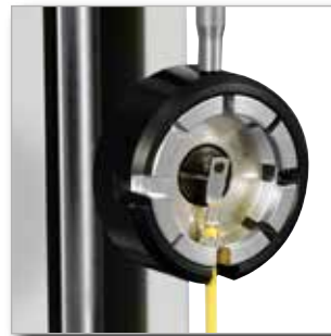
Crimp terminal tensile test
