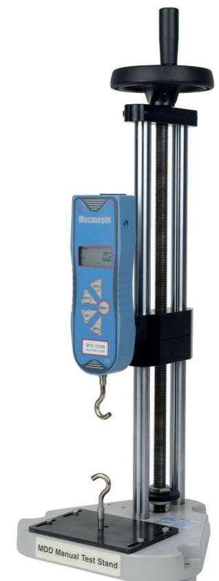
BFG shown mounted to the MDD manual test stand
