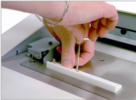
Secure the first rail; do not overtighten
