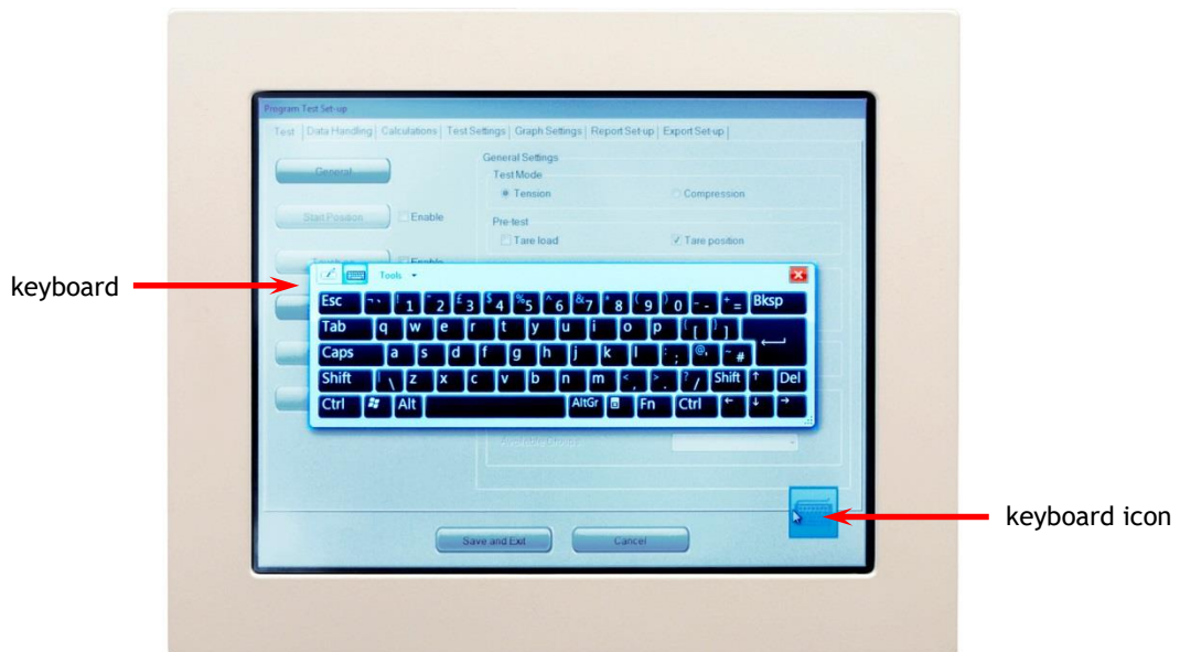
The FPT-H1- xt console showing the floating keyboard icon bottom right, and keyboard
