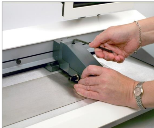
Attaching and removing the loadcell
