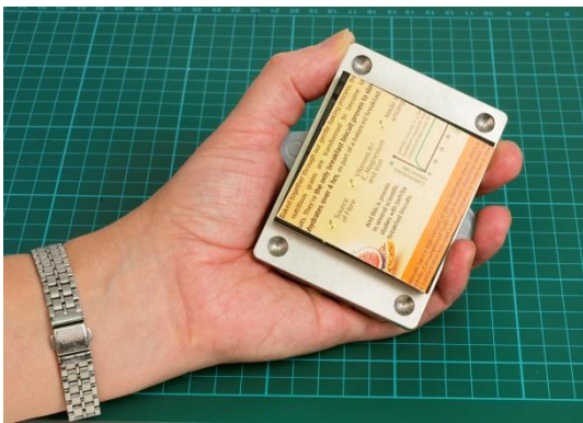
Sample not set square card edge projects, area not fully supported
