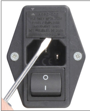
Removing the fuse carrier
