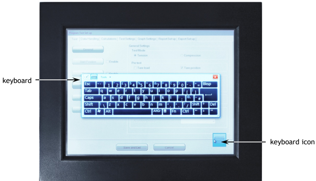
The - xt console showing the floating keyboard icon bottom right, and keyboard
