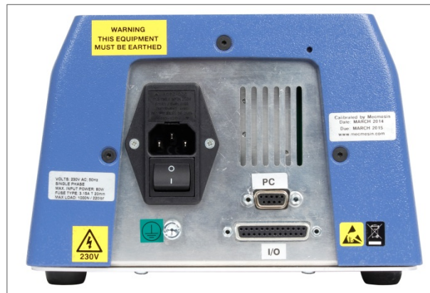
Helixa rear panel. Plug the data cable into the socket marked ‘PC’.
