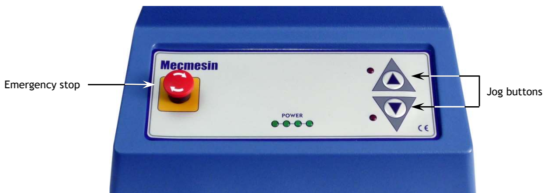
The front panel of the MultiTest 1- i . Vortex- i has a similar emergency stop button and clockwise and anticlockwise jog buttons.
