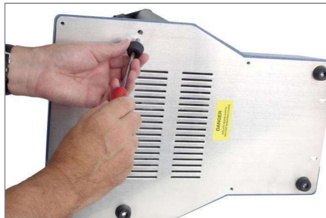
Fitting rubber feet to the base of the test stand
