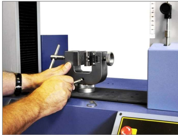
Attaching a grip with the QC Quick Interchange fittings
