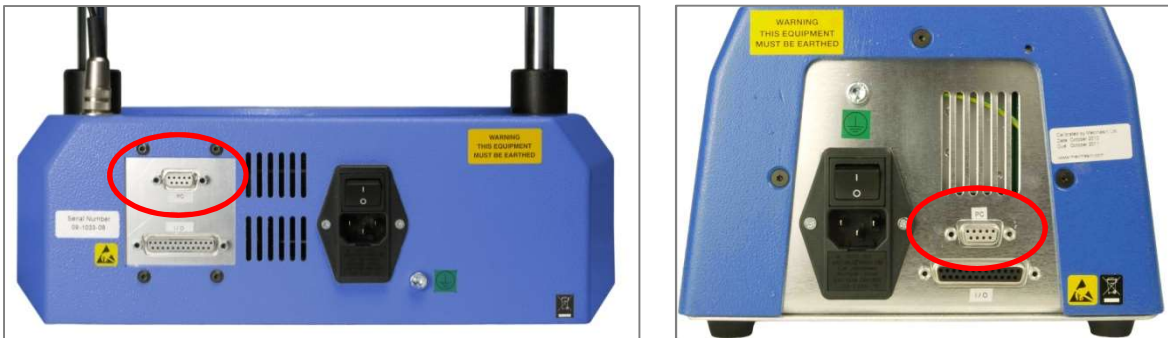
Rear panels of a Vortex- i (left) and MultiTest- i (right). Plug the USB cable into the circled PC socket.
