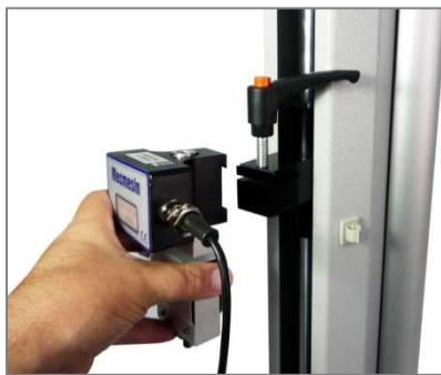
Slide the loadcell onto the dovetail ...
