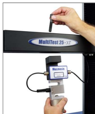
Attaching a loadcell on a twin-column system
