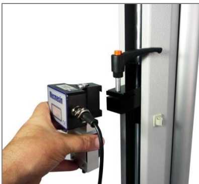
Slide the loadcell onto the dovetail ...
