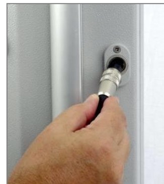
connect the loadcell
