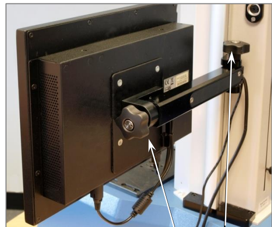
Use the two knobs to adjust tilt and swing
