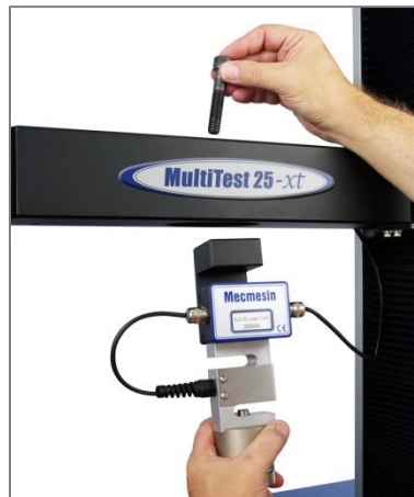
Attaching a loadcell on a twin-column system
