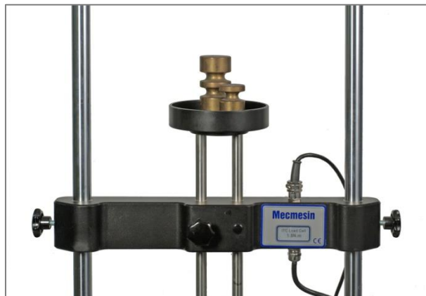
Crosshead fitted to Vortex-xt with top-load weights in the carrier
