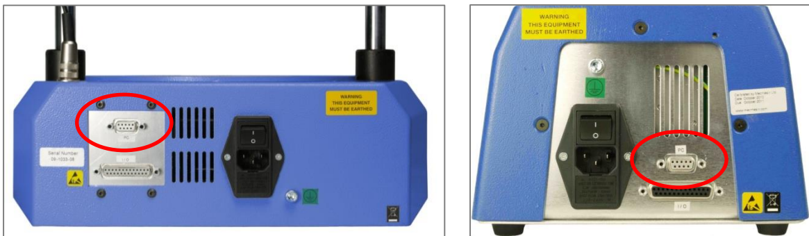
Rear panels of a Vortex-xt (left) and MultiTest-xt (right). Plug the USB cable into the circled PC socket.
