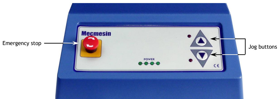
The front panel of the MultiTest 1-xt. Vortex-xt has a similar emergency stop button and clockwise and anticlockwise jog buttons.
