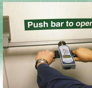
testing release force of safety bar
