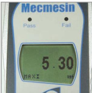
Mecmesin provides easy analysis tools to evaluate job tasks and the capabilities of personnel insitu. Where the task involves exertion over a given period of time, continuous measurements are recorded and the average force, over the time period, is automatically calculated in addition to the peak strength required to perform the task.
