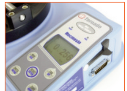
Digital Display Showing Maximum Release Torque. Slip and Bridge Values are also Available
